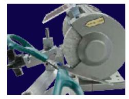
Hone scissors/shears to a razor sharp edge for more efficient cutting
